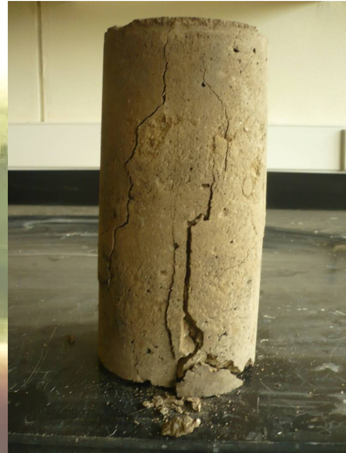
Failure of Cylinder in Tension
