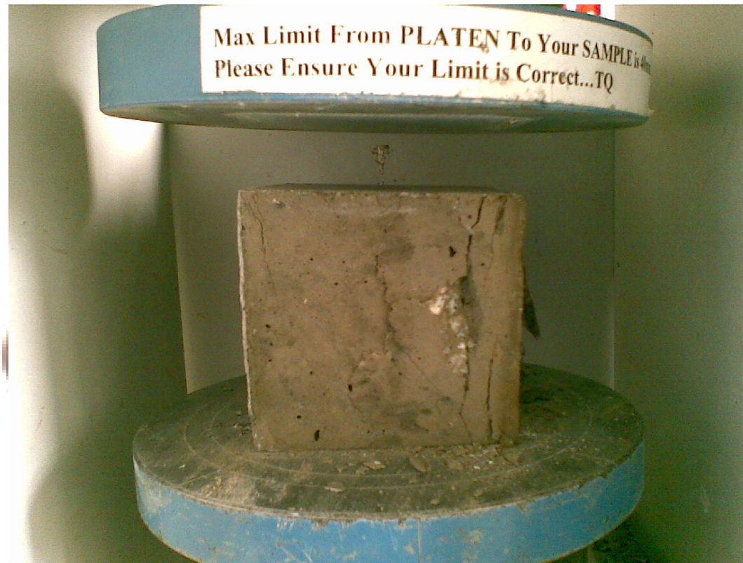
Failure of testing cube
