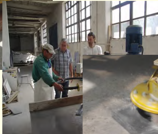
Turning motion of grinding stones
