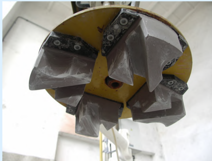
Semi-industrial grinding: Grinding stones fixed in holder
