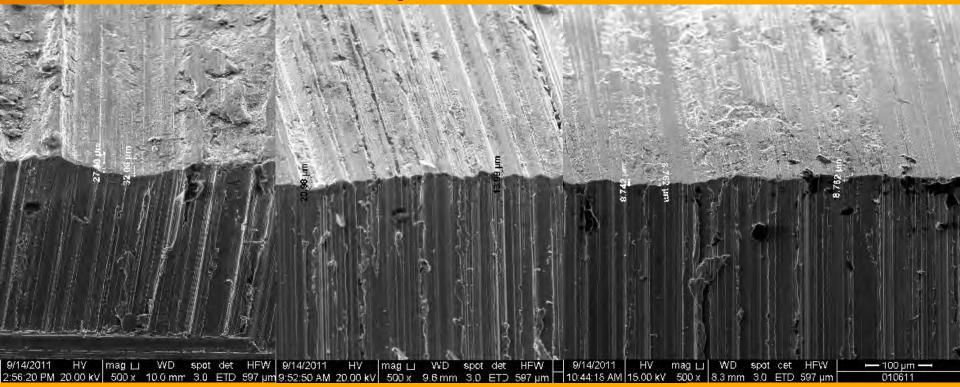
brown corundum F36 marks: 27.4 – 32 μm brown corundum F100 marks: 13 – 20.9 μm white corundum F500 marks: 8.74 - 8.76 μm
