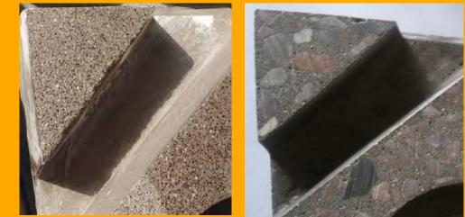
Detailed view on grinding stones after grinding
