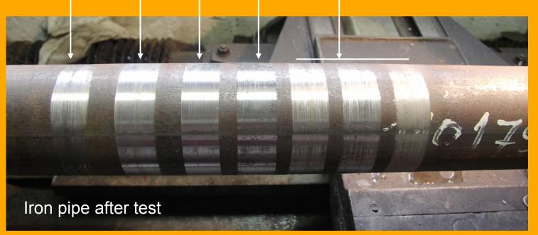
Different particle size of grains – different abrasive marks
