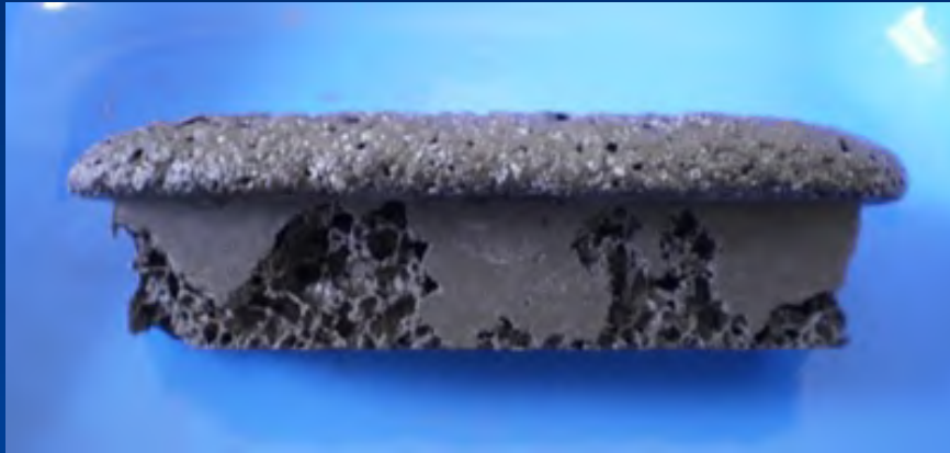
MSWI ash without pretreatment – test prism
