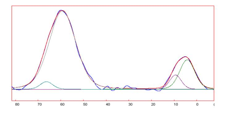
We could observe a typical shift from [6] Al to the dominantly [4] Al coordination which is indispensable for alkalization in aqueous solution.
