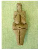
**a)** molding of a clay paste containing 2% by weight of NaOH powder and 30% water.
