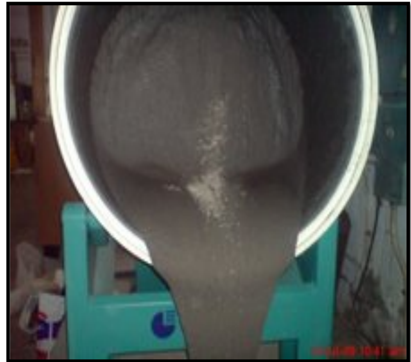
Flowable UHPC mix
