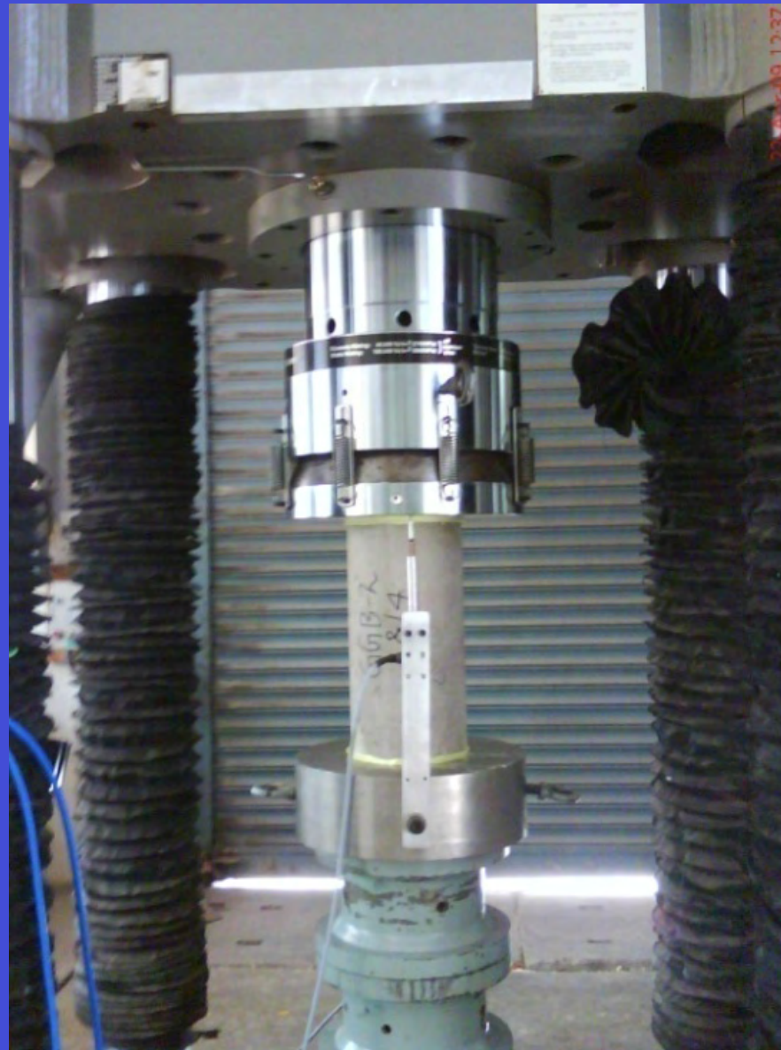
Test Set up for recording stress-strain curve
