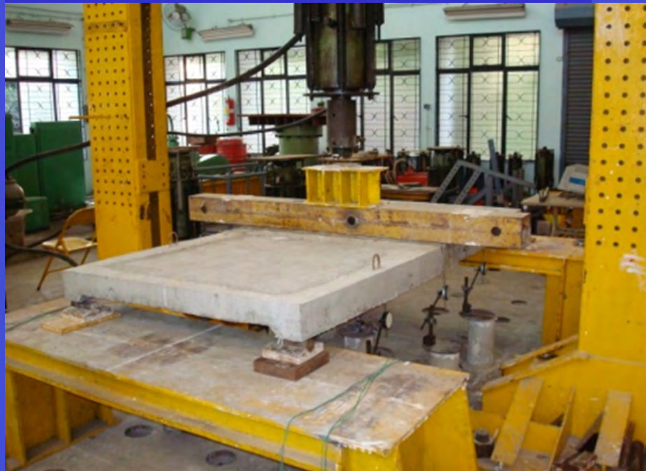
Testing of Slab with GPC Joint after 24 hours
