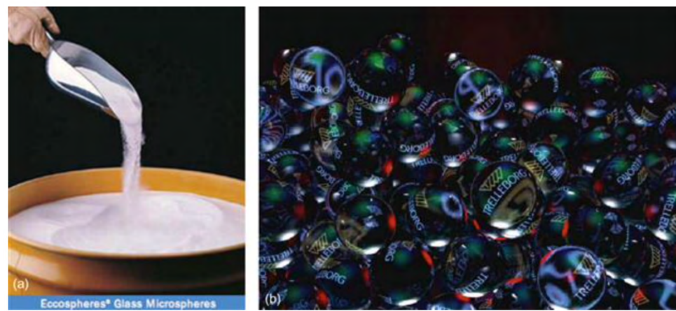
5.3 Macroscopic (a) as well as microscopic (b) views of glass microspheres. (Courtesy Trelleborg.)
