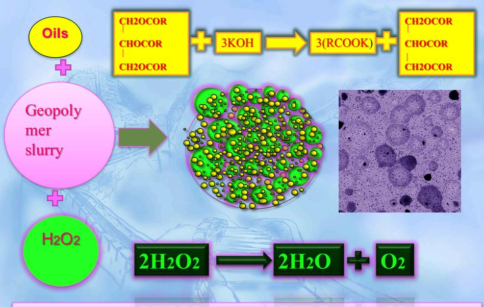
The mechanism of producing pores by saponification and peroxide combined routes
