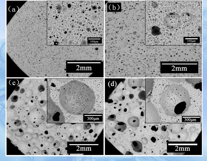
SEM images of MGFs produced using different amounts of hydrogen peroxide (a): y=0.0; b) y=0.05; c) y=0.10; d) y=0.15. x=0.20); the insets are a magnified view of a cell and surrounding struts. University of Padova-DII-Chengying Bai
