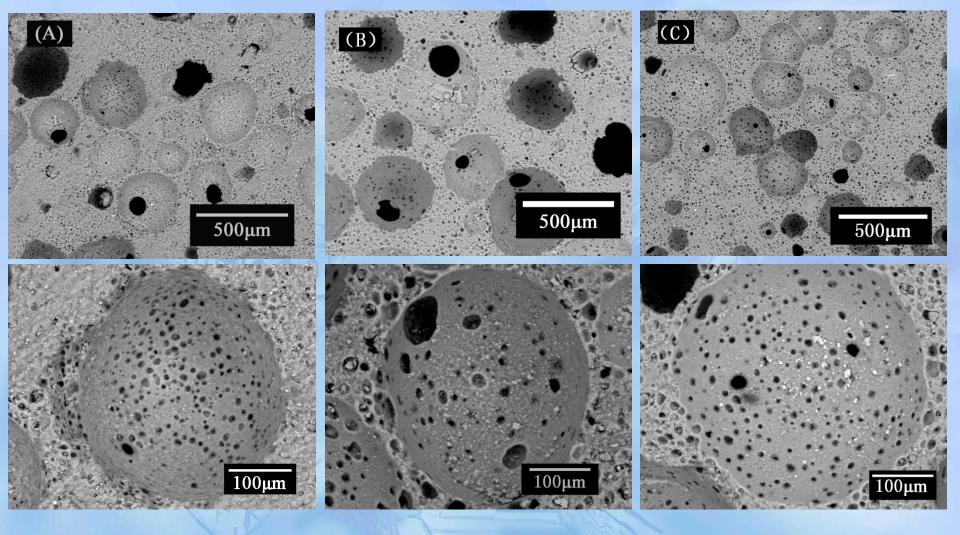
SEM images of MGFs produced using: canola oil (A); sunflower oil (B); olive oil (C). The below of figures (A)-(C) are a magnification of a cell to better visualize the cell windows. University of Padova-DII-Chengying Bai
