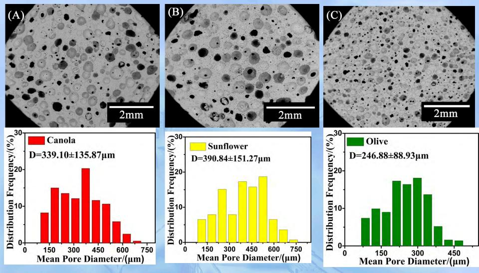
SEM images of MGFs produced using: canola oil (A); sunflower oil (B); olive oil (C). The below of figures (A)-(C) report the cell size distribution data. University of Padova-DII-Chengying Bai
