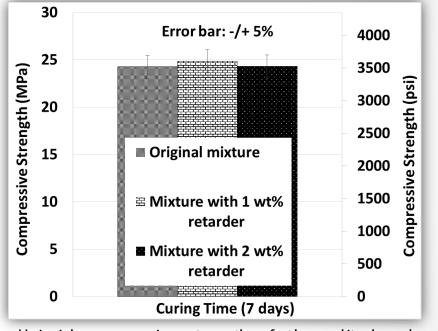
Uniaxial compressive strength of the aplite-based geopolymers cured at 90°C and 2000 psi.
