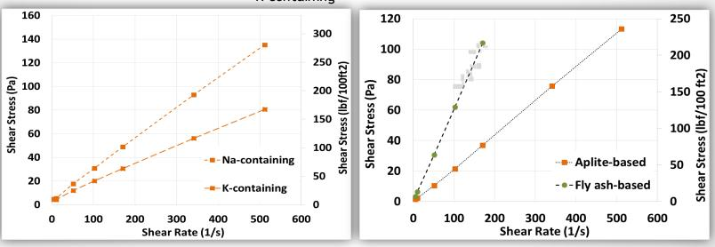
Shear stress vs. shear rate for Na- and K- containing aplite-based geopolymers at ambient condition.
