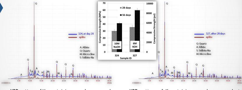
XRD pattern of Na-containing geopolymer cured at ambient temperature for 28 days.
