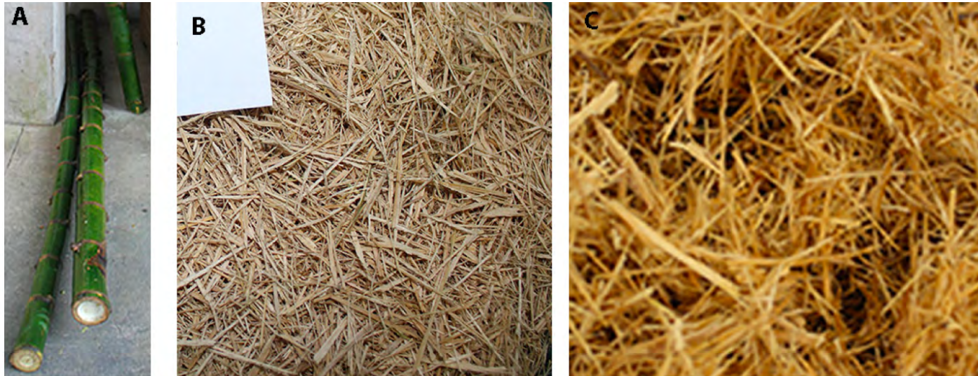
Figure 1. (A) Water-treated bamboo culms; (B) mechanically attained air-dried fiber bundles; (C) washed BF reinforcement just before use
