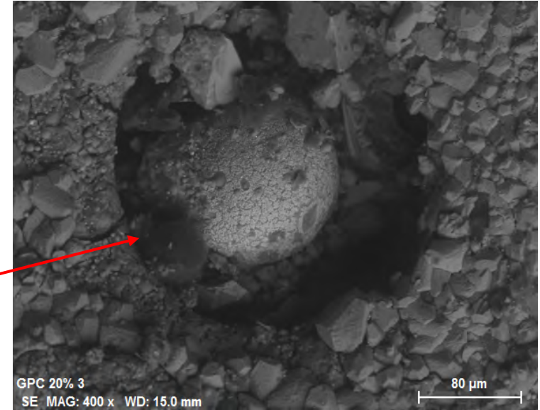
Poor bond and gap between GPC matrix and MPCM
