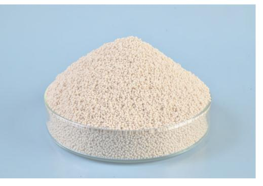
Introduction of micro active fillers based on natural raw materials will improve the properties of 3D geopolymer concrete, taking part in a reaction of geopolymerization, reduce the weight of the structure and reduce thermal conductivity of the building.
