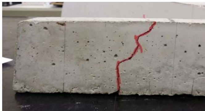
ULTIMATE POSITIVE MOMENT AT RAIL SUPPORT (FATIGUE TEST) FOR ORDINARY PORTLAND CONCRETE
