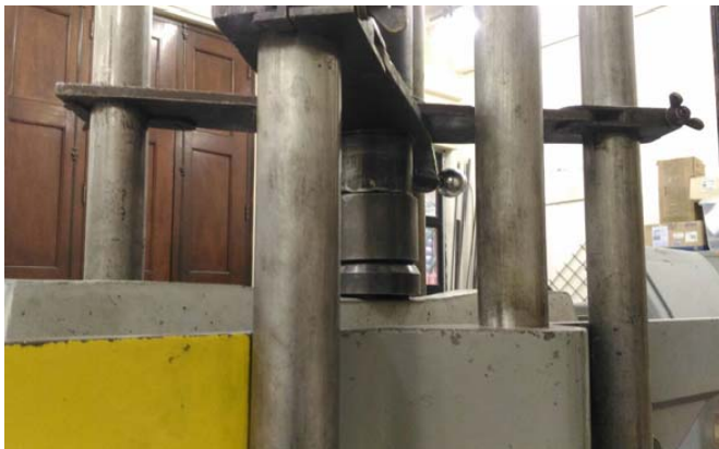
POSITIVE MOMENT AT MID-SPAN FOR GEOPOLYMERIC MICROCONCRETE
