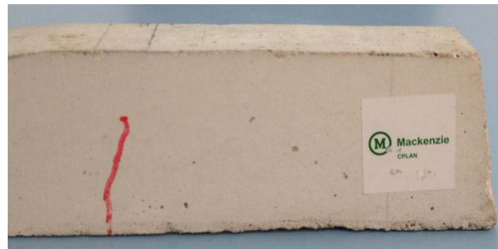
ULTIMATE POSITIVE MOMENT AT RAIL SUPPORT (FATIGUE TEST) FOR GEOPOLYMER MICROCONCRETE
