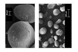
Feldspar : is produced from naturally occuring combination of alumina and silicate having mix oxides and no free crystalline silica. This material is hard and has angular particles that create a rigid reinforcing network.
