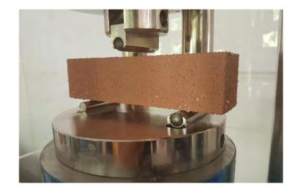
Tensile / Cold bending strength
