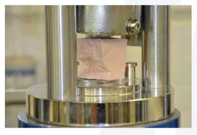
Compressive / Cold crushing strength
