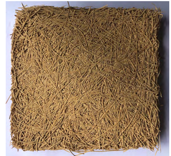
Troldtekt's acoustic panels produced with geopolymer-binder
