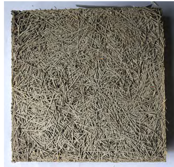
Troldtekt's acoustic panels produced with geopolymer-binder
