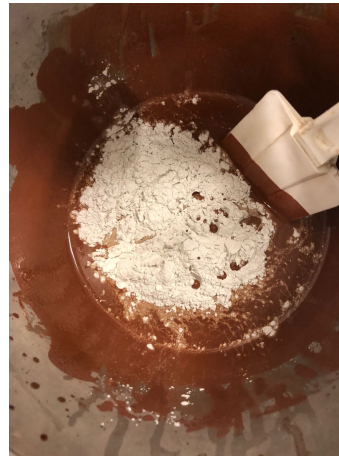
Add Slag which is most reactive so we add it at last for 3 mins
