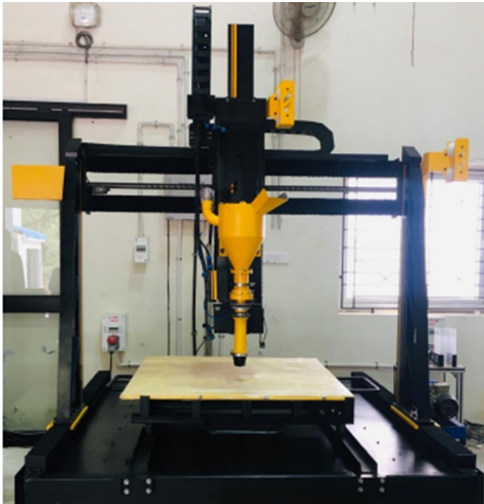
Extrusion based 3D concrete printer 1000 mm x 1000 mm x 500 mm
