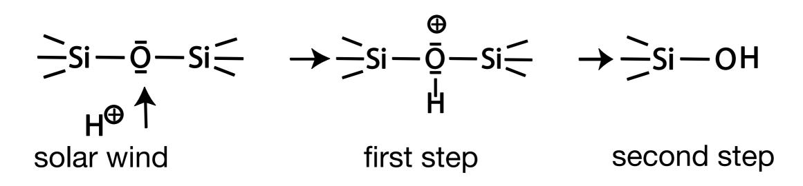
Solar-wind derived water on Moon Once formed, the OH is permanently bound to the lattice. This specific property is also found in our man-made geopolymers, where the chemically bound water is actually in the form of hydroxyl -Si-OH or -Al-OH structural units.
