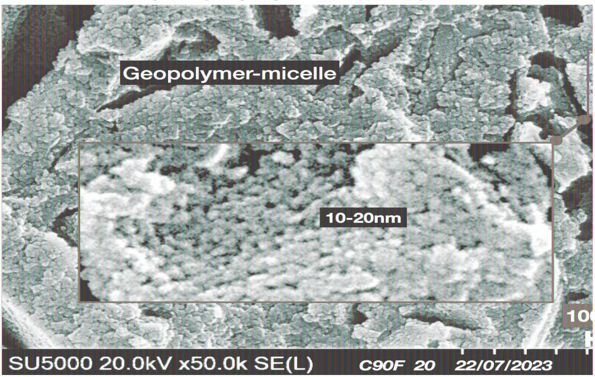
• X-ray diffraction and NMR analyses confirmed that the 3D-network of the poly(sialate) geopolymer micelle remains intact in vacuum.
