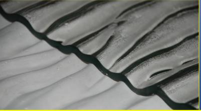
The detail of fussed glass coping mould nodulation, heated on 830°C with 25 minutes dwell.
