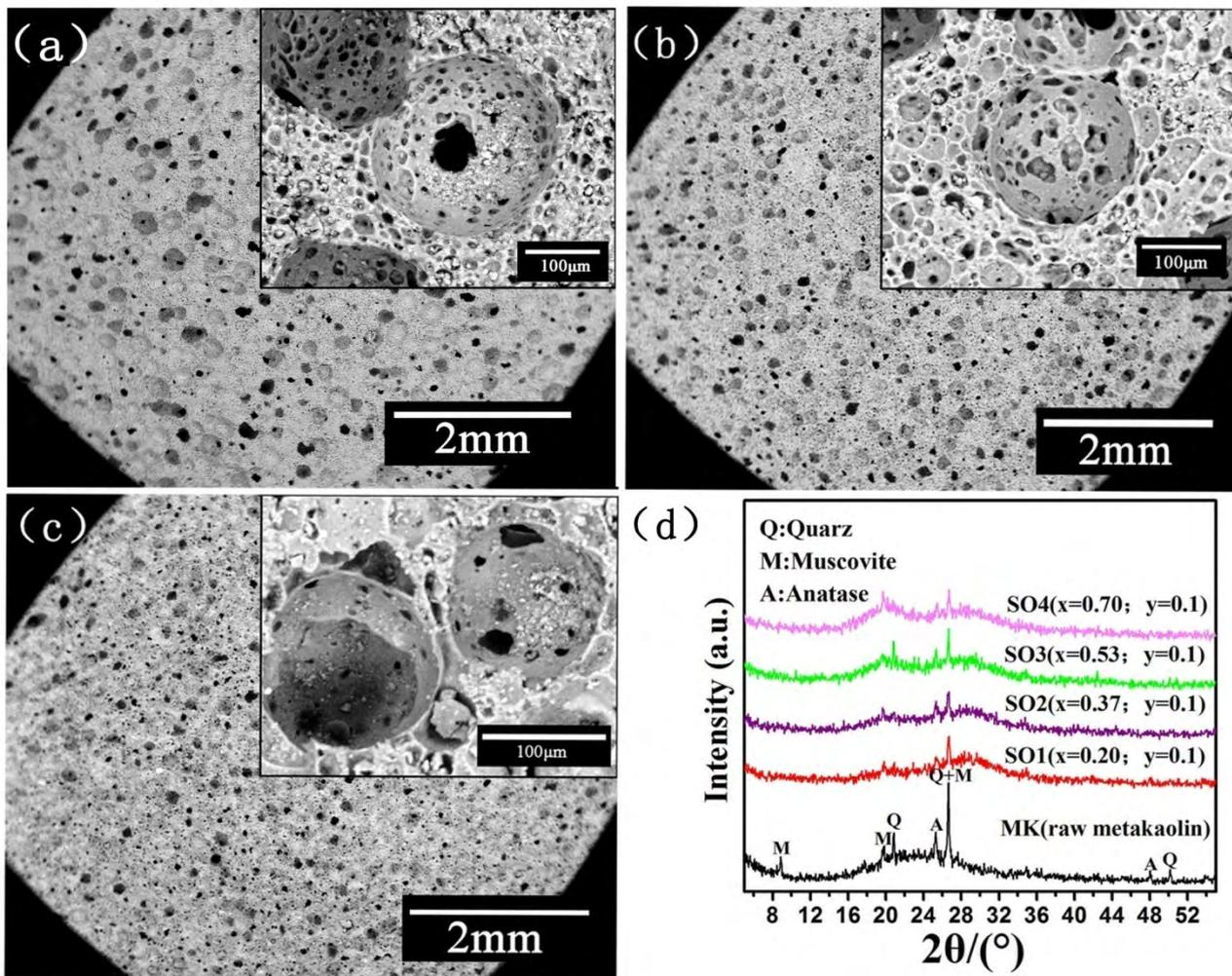
a-c) Morphology of MGFs produced with various amounts of olive oil (a)  $x=0.37$ ; (b)  $x=0.53$ ; (c)  $x=0.70$ ); insets show a magnified view of a cell and surrounding struts. d) XRD patterns of pure MK and of different samples.
