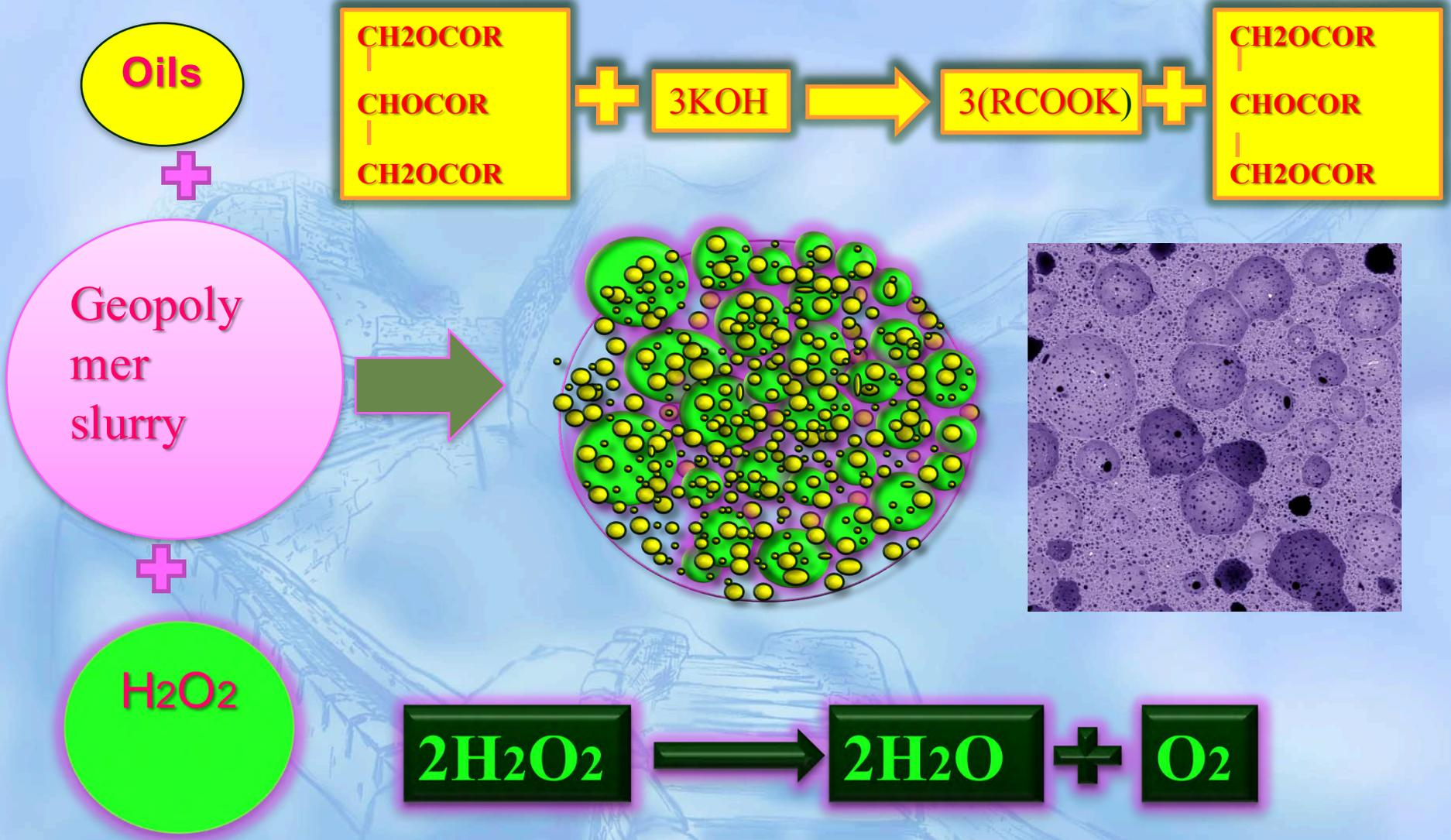
The mechanism of producing pores by saponification and peroxide combined routes
