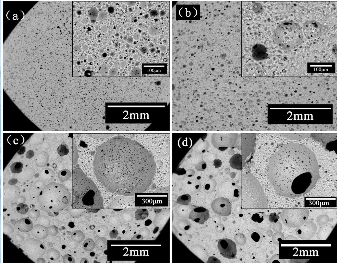
**SEM images of MGFs produced using different amounts of hydrogen peroxide (a):  $y=0.0$ ; b)  $y=0.05$ ; c)  $y=0.10$ ; d)  $y=0.15$ .  $x=0.20$ ); the insets are a magnified view of a cell and surrounding struts.**
