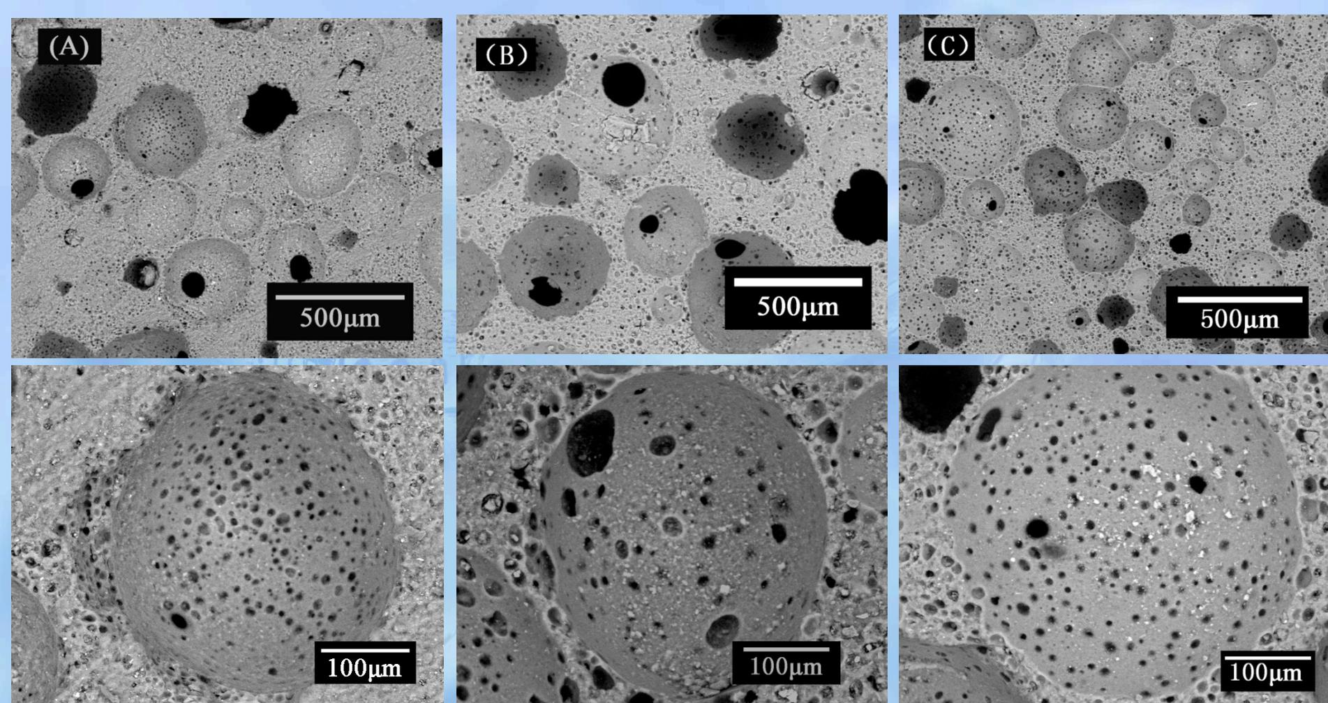
**SEM images of MGFs produced using: canola oil (A); sunflower oil (B); olive oil (C). The below of figures (A)-(C) are a magnification of a cell to better visualize the cell windows.**
