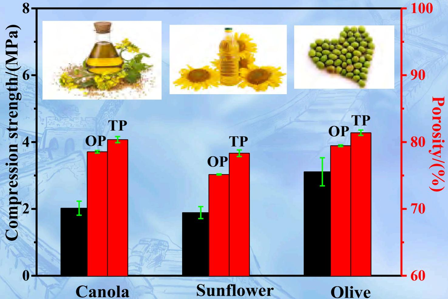
**Porosity and compression strength of MGFs produced using different types of oils (OP = open porosity (vol%); TP = total porosity (vol%)). Samples produced using  $x=0.2$ ,  $y=0.1$ . (Same content of oils and  $H_2O_2$ )**
