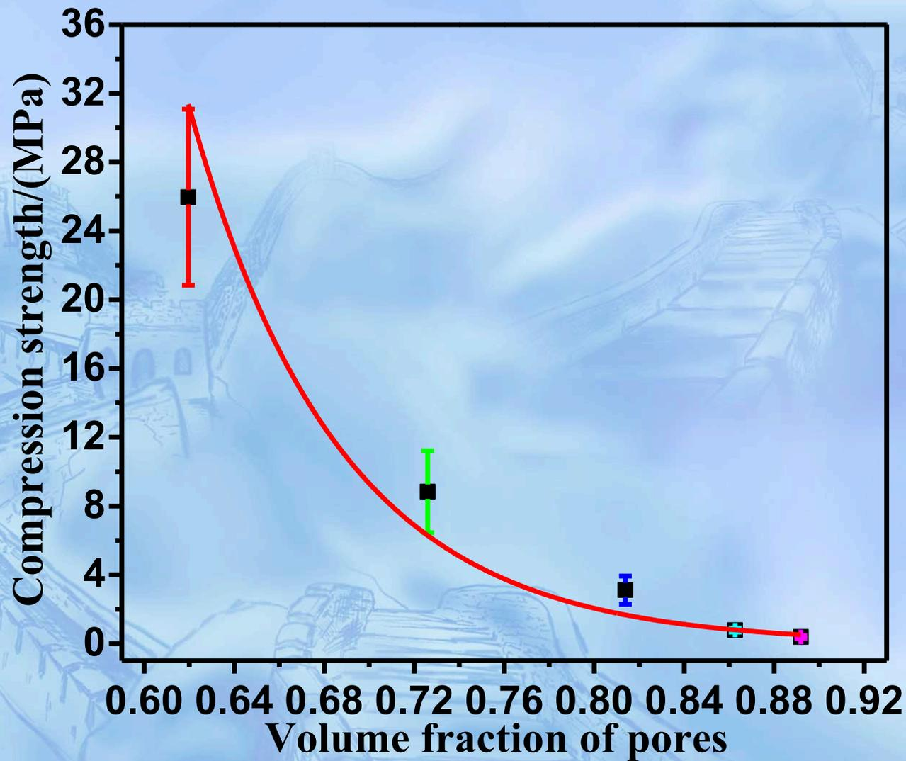
**Plot of compression strength vs. total porosity for MGFs produced using different contents of  $H_2O_2$  and the same amount of olive oil ( $x=0.20$ ).**
