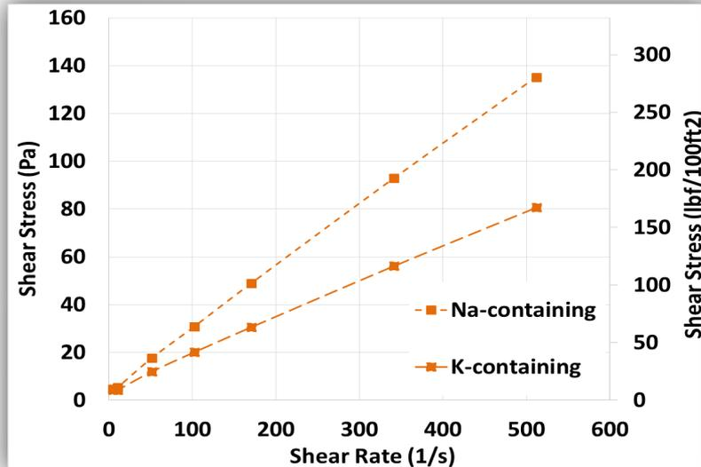
Shear stress vs. shear rate for Na- and K- containing aplite-based geopolymers at ambient condition.
