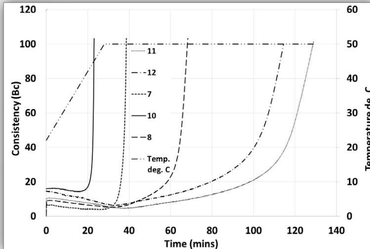
Atmospheric consistometer of the aplite-based geopolymers with different mix ratios.
