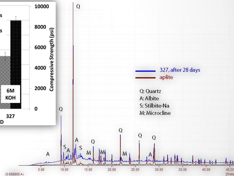
XRD pattern of K-containing geopolymer cured at ambient temperature for 28 days.
