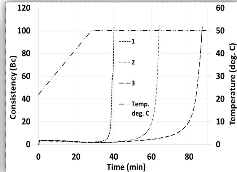
Atmospheric consistometer of the aplite-based geopolymers with different dosages of retarder.
