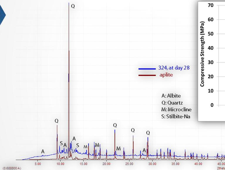
XRD pattern of Na-containing geopolymer cured at ambient temperature for 28 days.
