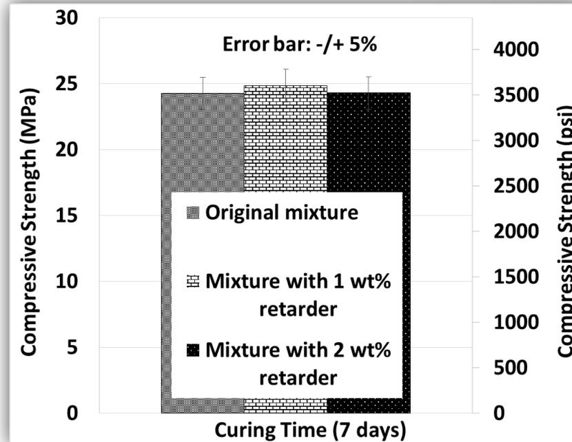
Uniaxial compressive strength of the aplite-based geopolymers cured at 90C and 2000 psi.
