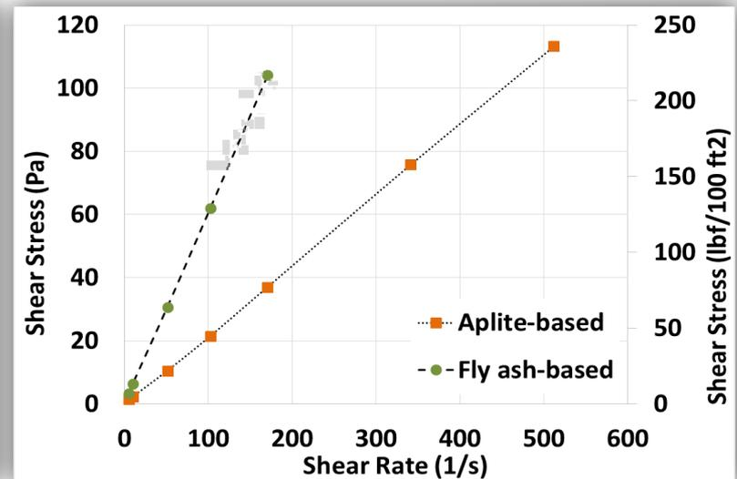
Shear stress vs. shear rate for fly ash- and aplite-based geopolymers at ambient condition.
