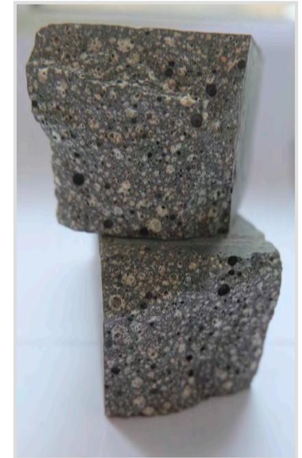
Introduction of micro active fillers based on natural raw materials will improve the properties of 3D geopolymer concrete, taking part in a reaction of geopolymerization, reduce the weight of the structure and reduce thermal conductivity of the building.
