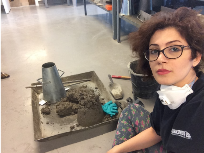
A failed slump test of a geopolymer concrete
