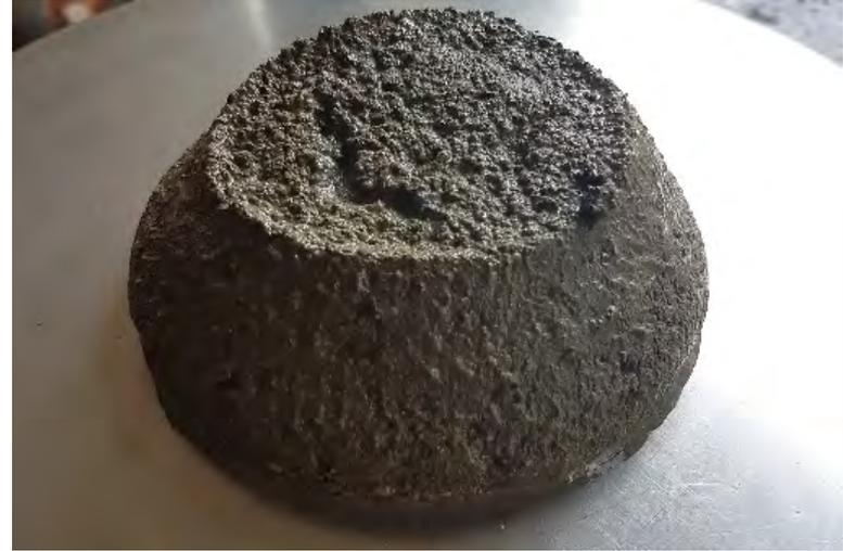
Concrete slump test
