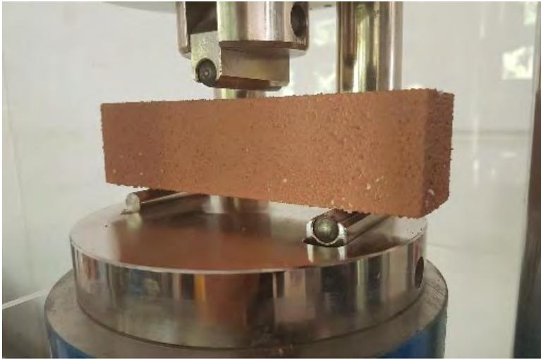
Tensile / Cold bending strength
