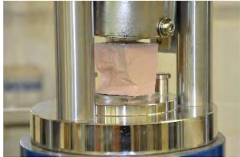
Compressive / Cold crushing strength
