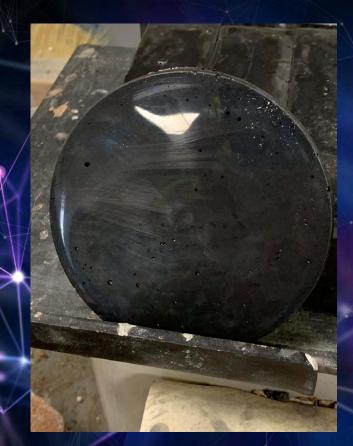
Patent Pending Geopolymer coating for thermal conductivity and thermal insulation
