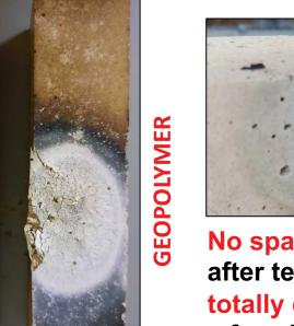
**No spalling immediately** after tests, but Portland totally collapses after a few days.
