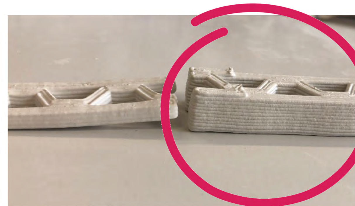
Incorrect curing process -VS- Good post-processed curing
