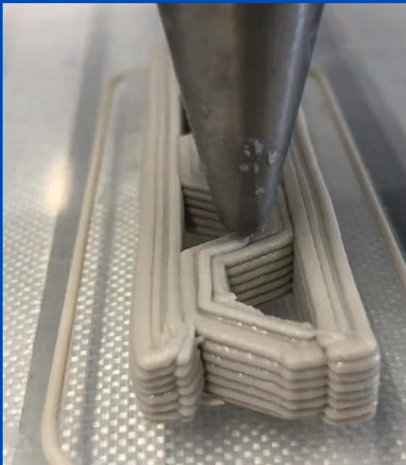
Controlled layer flow Nozzle Diameter = 1mm
