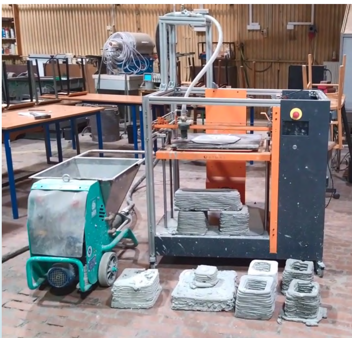
Small-Scale concrete 3D printer.
