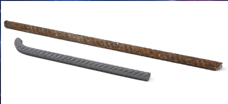
COVERING AND PASSIVATING RUSTY REBARS
