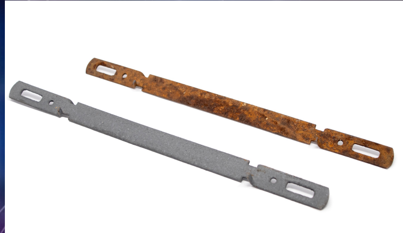
PASSIVATING EFFECT ON RUSTY IRON ELEMENTS
