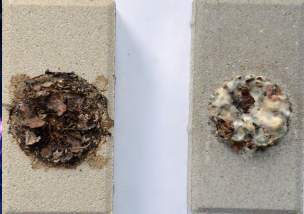
MATTER + VS OPC Std. After 28 d of mold growth
