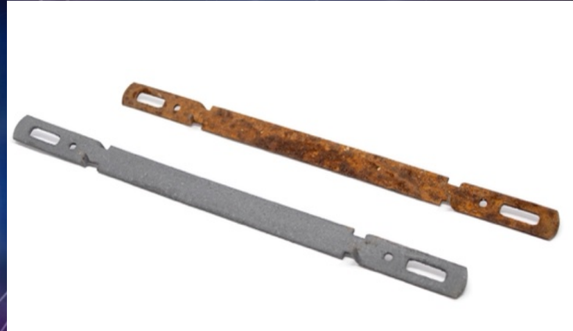
PASSIVATING EFFECT ON RUSTY IRON ELEMENTS
