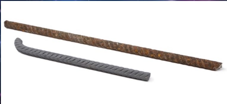
COVERING AND PASSIVATING RUSTY REBARS
