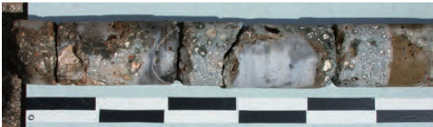
Fig. A3.8: PCO.2003.01, detail, 0 to -0.58 m. Pumiceous tuff and gray limestone caementa , and mortar with relict lime clasts and possible clots of relict lime putty.
