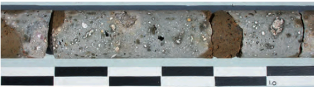
Fig. A3.9: PCO.2003.01, detail, -0.50 to -1.10 m. Pumiceous tuff caementa and pumiceous mortar with abundant lime clasts.
