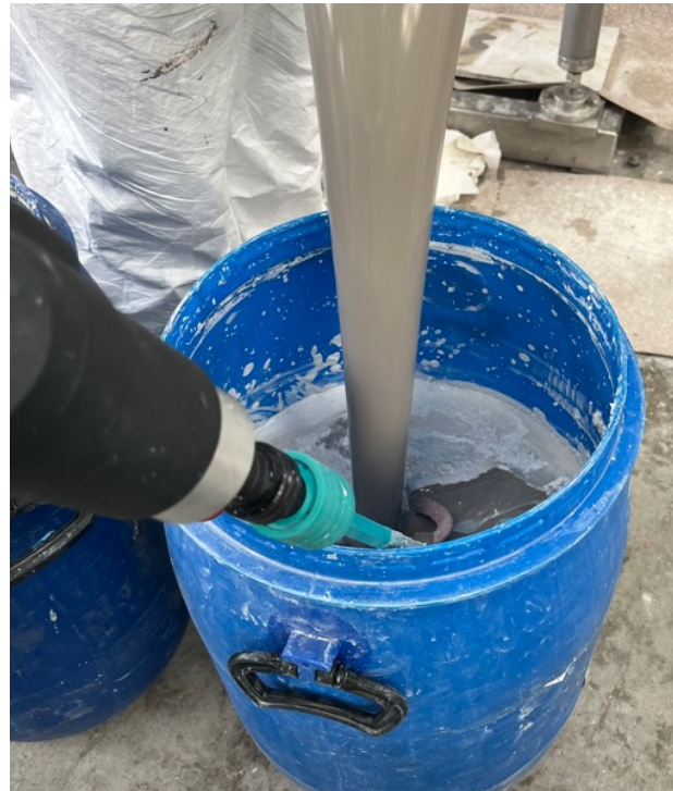
02 Slurry added to Magnox sludge paste
