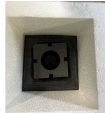
Graphite block (M2) in mould
