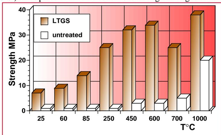
L.T.G.S. may dramatically enhance and modernise the traditional ceramic industry. Once geopolymerised into PCDS (Na-poly(cyclodisialate) or PCTS (K-poly(cyclotrisialate), at 125-250°C, ceramic bodies may be ultra rapidly fired at 1000°C-1200°C, to produce high quality ceramics (Fig. 15)
