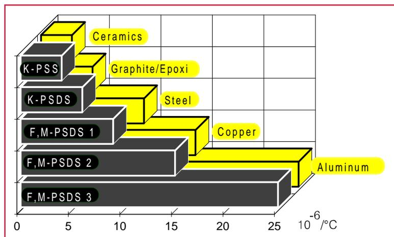
Geopolymite resins are designed to match the CTE of steel, enabling them to be used with steel inserts or frames, or have a CTE matched to that of other metal, carbon-fiber/epoxy parts, or any organic resins.
