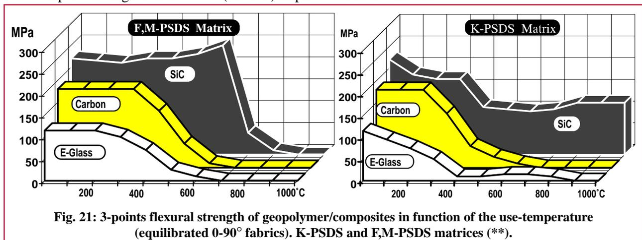
Fig. 21: 3-points flexural strength of geopolymer/composites in function of the use-temperature (equilibrated 0-90° fabrics). K-PSDS and F,M-PSDS matrices (\*\*).
